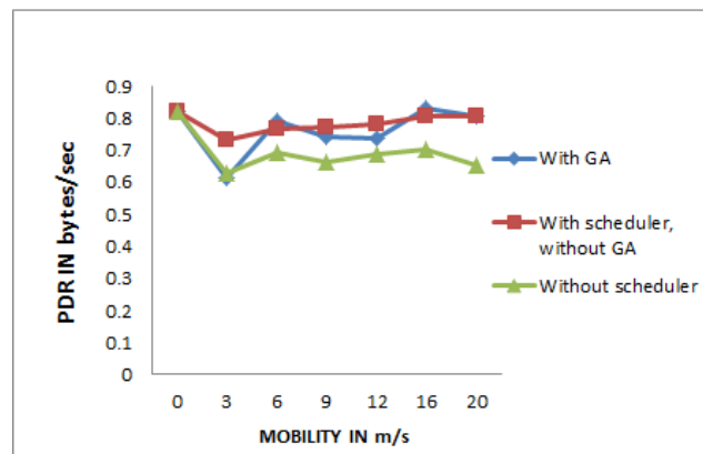
Graph 1. Packet Delivery Ratio Vs Mobility (with DSR)
