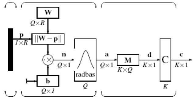
Fig. 5 PNN structure, R: number of features, Q: number of training samples, K: number of classes.
