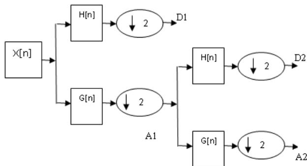
Fig. 3 Two level wavelet decomposition
