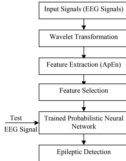
Fig. 1 Data flow diagram of the proposed system
