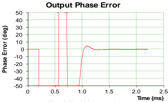
Fig. 13 The PLL output phase error
