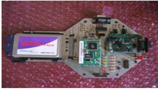
Fig. 1: EZL-80 PCMCIA-TTL interface with PCMCIA card
