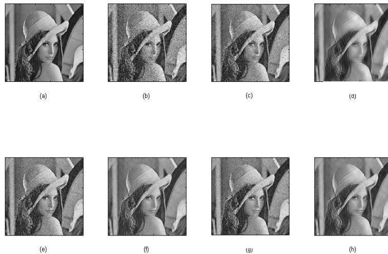
Figure 2. Denoising of Lenna (a) Original image. (b) Noisy image. (c) Soft thresholding using wavelets. (d) Multiple local soft thresholding using curvelets. (e) Hard thresholding using wavelets. (f) Multiple local hard thresholding using curvelets. (g) Multiple local cubic thresholding using wavelets. (h) Multiple local cubic thresholding using curvelets
