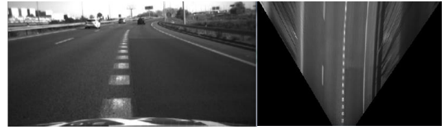
Fig. 1. Homographic transformation from road image into bird view and road lines detection.
