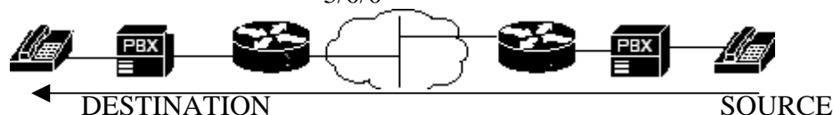
Figure (3) Linking PBXs over the IP Network (Local Dial Peers)
