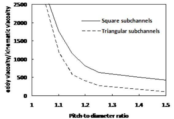
Fig. 6. Effect of pitch-to-diameter ratio on eddy viscosity,  $Re = 100000$
