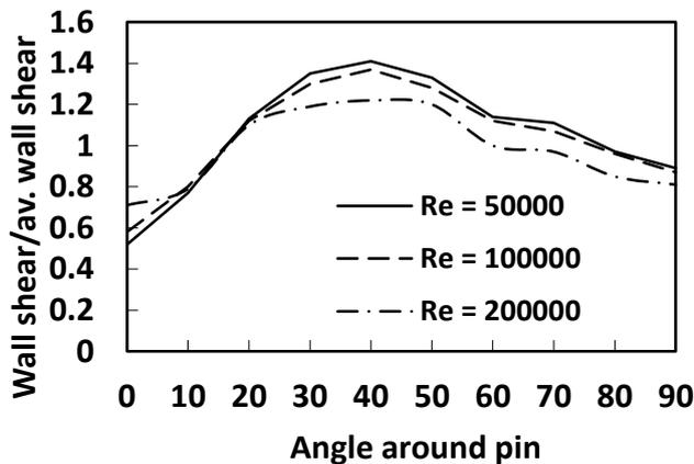
Fig. 4. The wall shear around rod,  $\gamma_p = 1.1$
