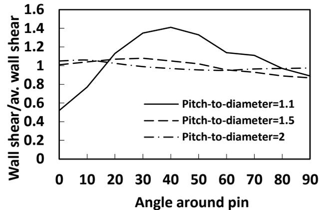
Fig. 5. The wall shear around rod,  $Re = 50000$
