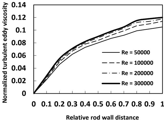
Fig. 7. Normalized eddy viscosity at different Re,  $\gamma_p = 1.1$
