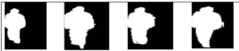
Fig.2: Image of person 1 after applying OR on 50 images for each state of gait of person1 for angle 90°
