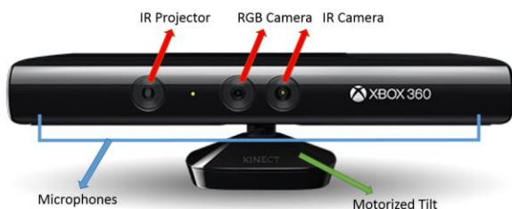
Fig. 1. Microsoft Kinect Sensor v1.
