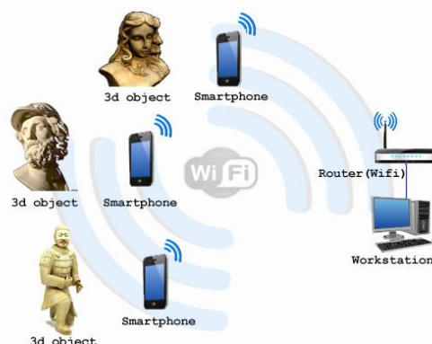
Fig. 4. The architecture of distributed 3D objects recognition system using smartphones.
